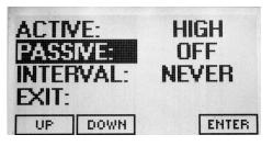
Press ENTER and then UP or DOWN to change the BACKLIGHT setting in the right column. Press ENTER to save the setting and return to the left column.
