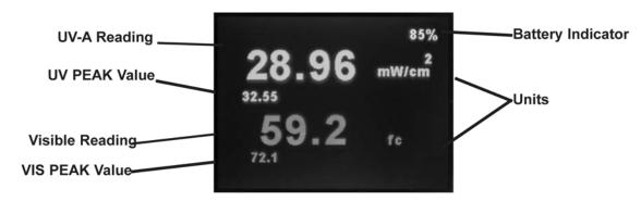
4. Three buttons control all functions of the AccuPRO and AccuPRO Plus. Simply press the **DOWN** arrow to reset the stored PEAK value (highest reading recorded since the last reset) across all measured wavelengths.
