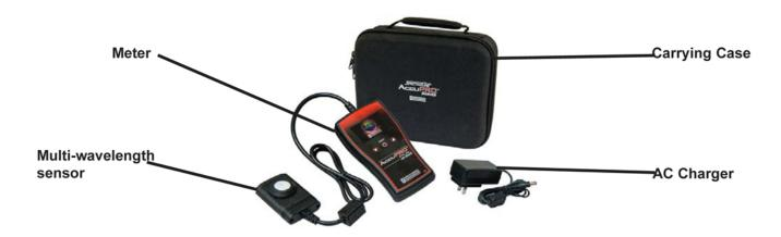
3. The AccuPRO automatically opens in **OPERATION** mode (see screen below) and begins to take readings. Shine the light (UV, VIS or Blue [XP-4000 only]) directly over the sensor. The meter will instantly read and display the light level for each wavelength (intensity/unit area). If using the AccuPRO Plus, press the **UP** arrow to toggle to blue light mode.
