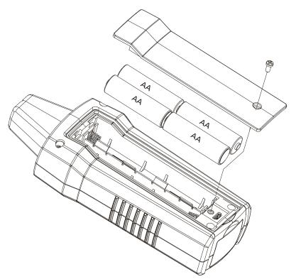
Figure 5.1: Changing the Receiver batteries
