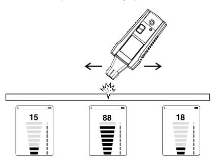
Figure 4.1: Using the Receiver to find a leak
