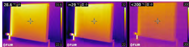
Figure 33.4 Images from a FLIR T440 with temperature ranges of -20 to +120^{\circ}\text{C} , (left, -4 to +248^{\circ}\text{F} ), 0 to +650^{\circ}\text{C} (middle, +32 to +1202^{\circ}\text{F} ) and +250 to +1200^{\circ}\text{C} (right, +482 to +2192^{\circ}\text{F} ). All other settings are unchanged.
