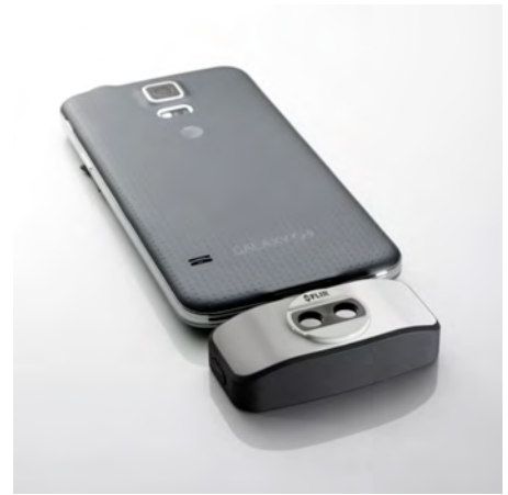
Figure 30.3 2015: FLIR One, an accessory to iPhone and Android mobile phones. Weight: 90 g (3.2 oz.).
