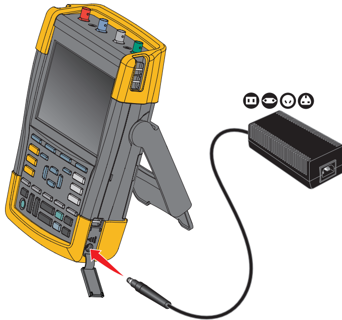
Figure 46. Charging the Batteries
