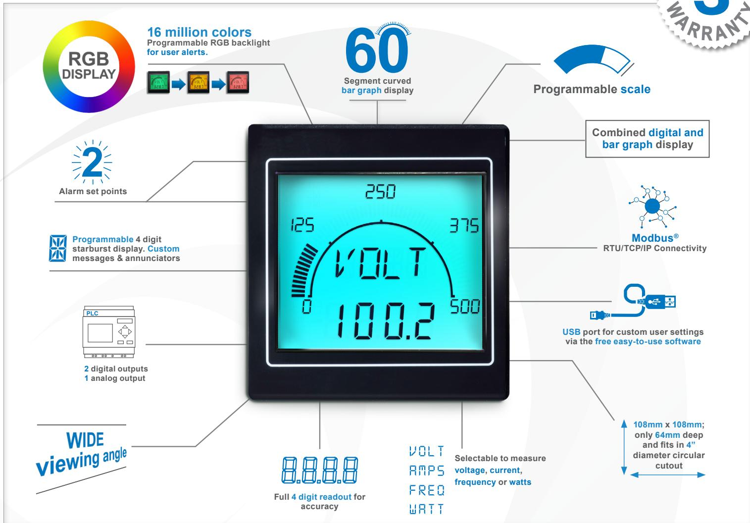
Designed for a wide range of power monitoring applications, the APM-MAX combines the instant visual representation of an analog meter with the speed and accuracy of a digital meter for instant recognition and precision measurement. The large 81.5mm x 66mm display features a two-line display, programmable scale, alarm set-points and color-changing, full color RGB backlight for instant alerts.
