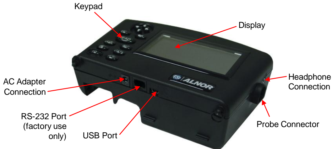
Figure 1: Features of the EBT730/EBT731 Micromanometer, Front View
