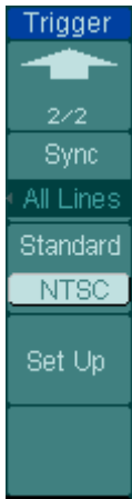
Figure 2- 59 Table 2- 35 The Alternate menu (Trigger Mode: Video, All Lines, Odd Field or Even Filed, Page 2/2)
