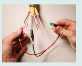
GREEN LED means wiring is properly identified.
