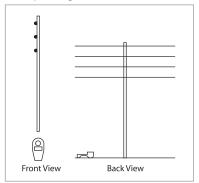
When taking wire measurements, ensure that there are no walls or buildings within a distance of 2 m (7 ft) either side of the meter, as reflections from these will distort the readings. Also ensure there are no trees or similar overhanging objects in the vicinity.
