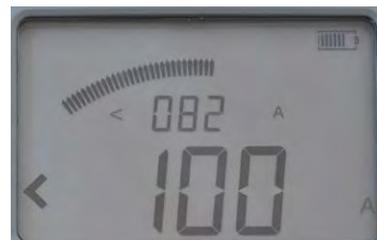
The maximum test current was 82 A and the test current was below 100 A.
