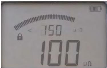
Here P/F limit was set to 150  $\mu\Omega$  and the measured resistance value is 100  $\mu\Omega$ .
