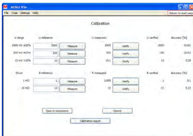
Figure 8.7.4 Ammeter calibration.
