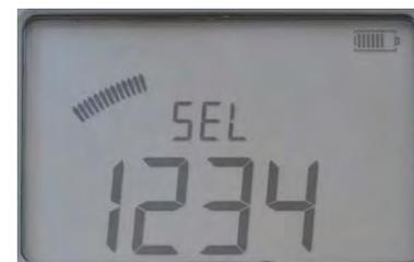
The measurements are numbered in numerical order (1 to 1999)
