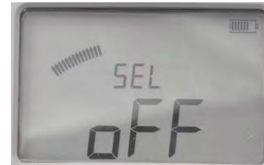
When the log is OFF only the latest value is stored and only until the performance of a following measurement, which overwrites the previous one.
