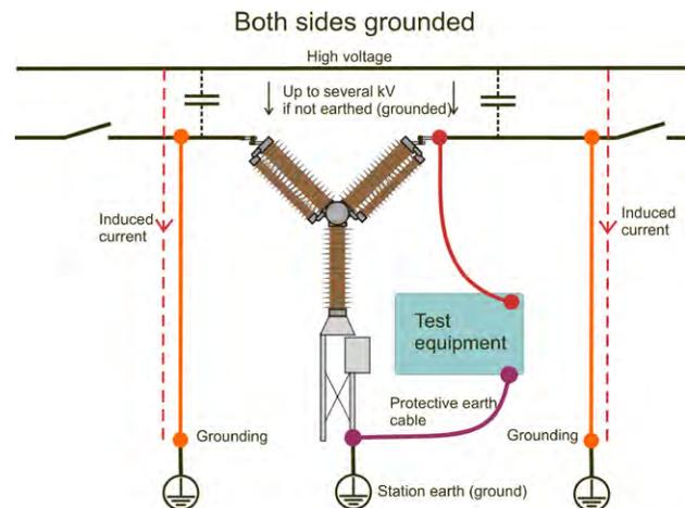
With both sides grounded the induced current will not pass through the test instrument.
