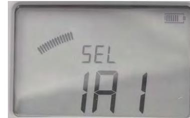
This mode is primarily designed for measurement on circuit breakers. The three characters (1A1) are supposed to indicate: Breaker, Phase, Interrupter.
