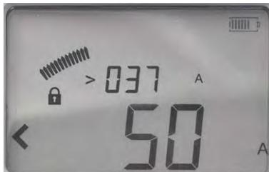
Picture shows an example after a measurement. The I min limit "50 A" has not been achieved, indicated by the ">" character to the left.
