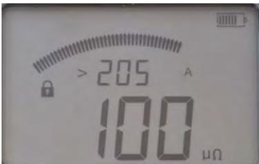
Min current during test was 205 A
