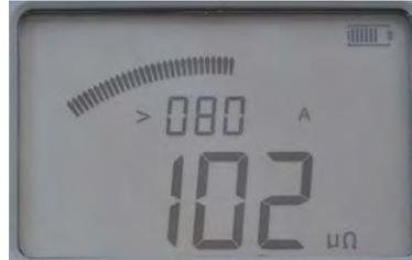
The minimum current was 80 A and the resistance value is 102  $\mu\Omega$ .
