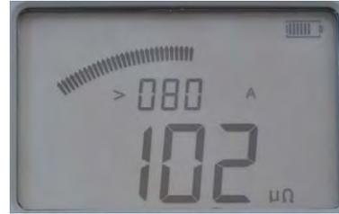
The minimum test current was 80 A and resistance is 102  $\mu\Omega$ .
