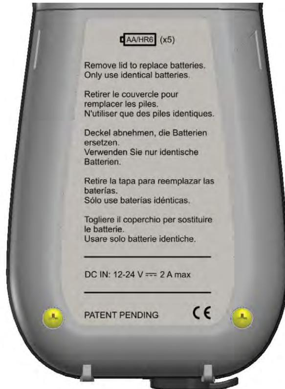
Loosen the two screws that holds the battery lid at the back of MOM2.
