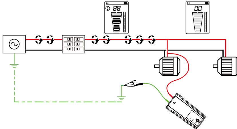
Figure 3.1b: Connecting Transmitter to Energized working system
