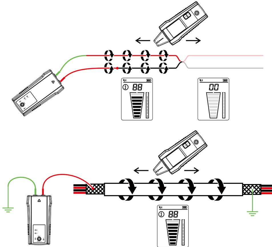
Figure 2.2b: Generating a signal in Loop mode
