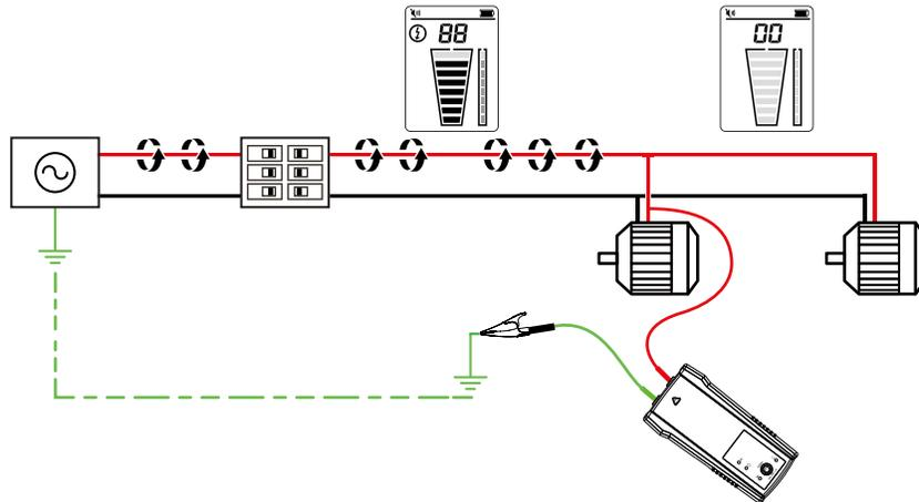
Figure 3.2c: Connecting Transmitter to Energized working system
