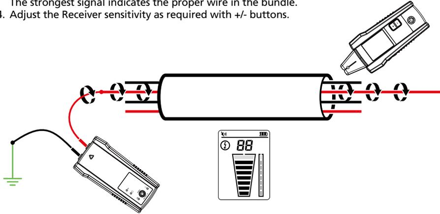
Figure 4.9: Identifying a specific wire in a bundle
