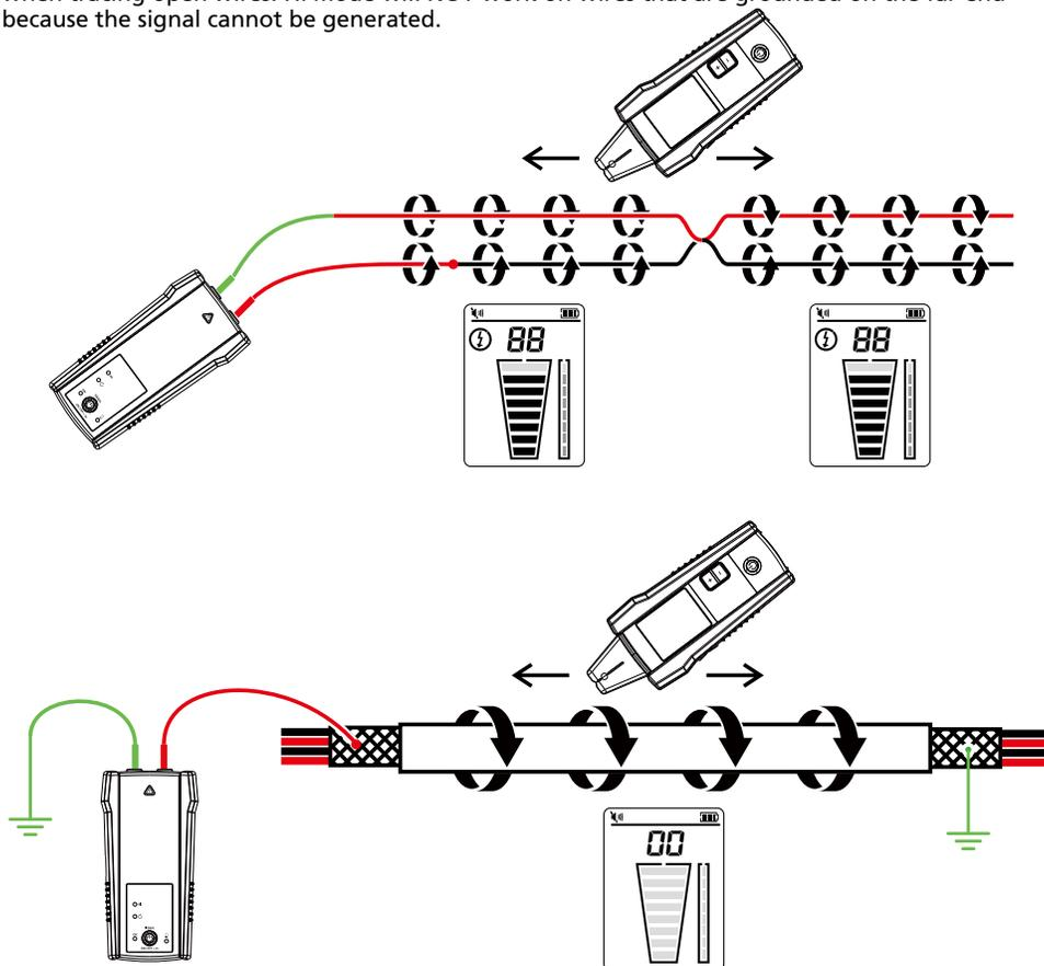
Figure 2.2a: Generating a signal with HIGH mode
