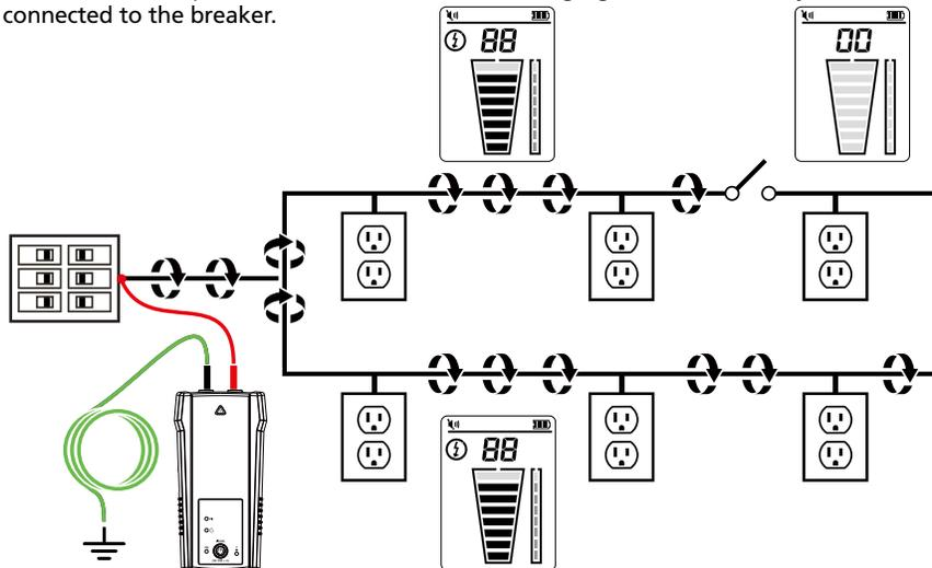
Figure 4.10: Mapping a circuit using test leads connection
