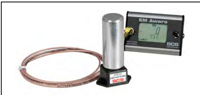
Figure 2. SCS 770066 EM Aware Monitor with ionizer antenna
