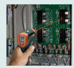
Max hold indicates and holds the peak temperature for easy identification of hot spots
