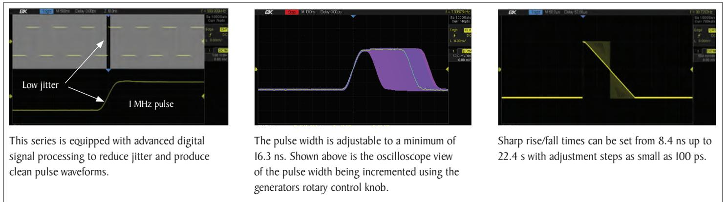
This series is equipped with advanced digital signal processing to reduce jitter and produce clean pulse waveforms.
