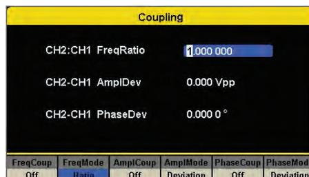
Customize channel coupling using frequency, amplitude, and phase. Enable automatic tracking between channels using deviation or ratio.
