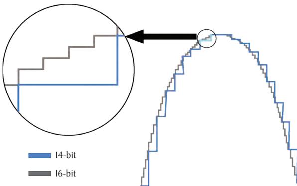
The 4060B Series uses 16-bit sampling for enhanced resolution resulting in lower distortion and more accurate waveforms.
