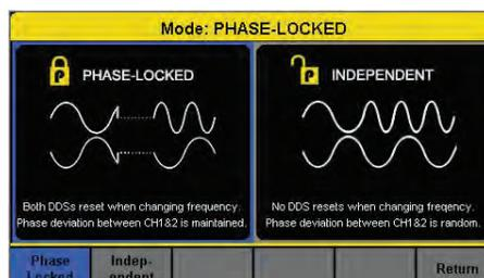
Phase-lock maintains phase deviation over both channels. In independent mode, the phase deviation between CH1 and CH2 changes at random allowing for smoother frequency transitions.
