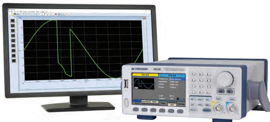
The provided waveform editing software can be used to create point-by-point arbitrary waveforms via freehand or waveform math functions. The standard LAN and USBTMC-compliant interfaces on the rear panel allow users to easily interface with a PC to load these waveforms into internal memory. The front panel also offers a convenient USB host port to save/recall instrument settings and waveform files on a USB flash drive.
