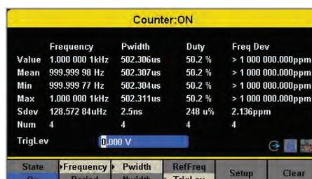
Displays mean, min, max, and many other frequency characteristics with an input frequency range of 0.1 Hz to 200 MHz.
