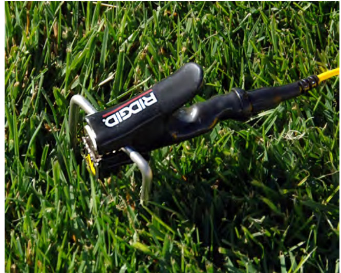
Figure 5 – Connecting the ST-305 Ground Stake
