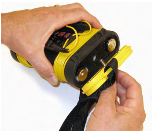
Figure 4 – Removing the Battery Cover
