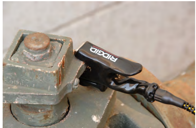
Figure 6 – Connecting the ST-305 using the clip
