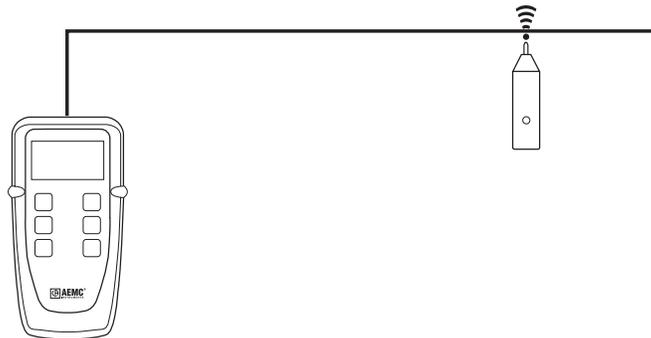
Pressing the **TDR /
