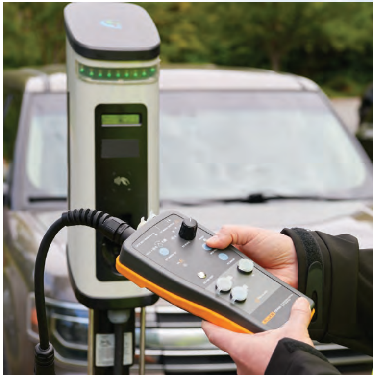
Fluke FEV-100 for e-mobility applications
