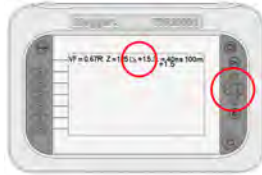
Adjust DDG. Single press increments by 0.1 dB Press and hold increments by 0.5 DB
