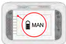
Current operational state. Currently in Manual operation
